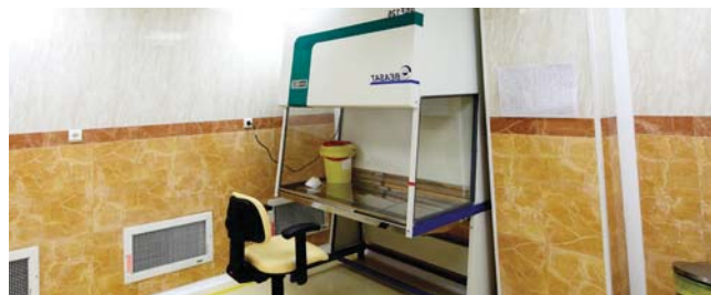
The Laminar Air Flow Cabinet for the preparation of Chemotherapy Drugs
